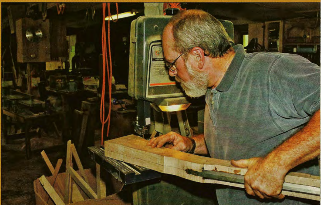
Top, both a gas and a coal forge (shown) are used by the gunmaker. Above, Haarer cuts out the stock pattern for his next flintlock.
