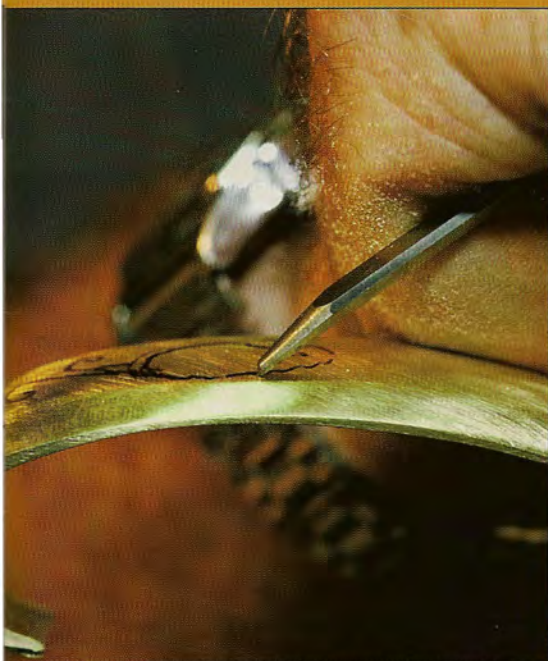
Lowell hand chisels the engraving on his flintlocks.
