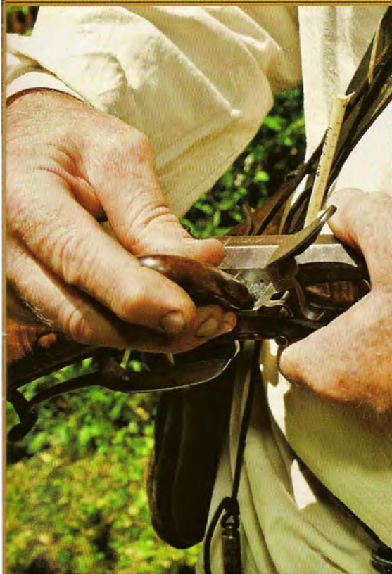
Lowell Haarer takes aim with one of his creations, above. Left, he primes the gun by putting a little powder in the flash pan. That aids in setting off the explosion needed to propel the shot or bullet.
