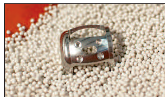
A main reel case is being polished by tiny ceramic beads.
